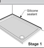
Once the walls have been tiled but **before** the enclosure is installed, the tiles **must** be silicone sealed to the tray all of the way around in one continuous bead.
