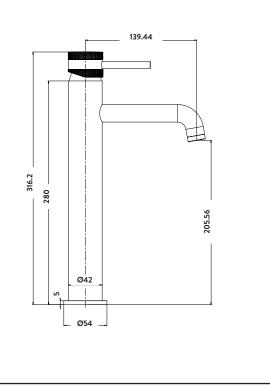
Dimensions (measurements in mm)
