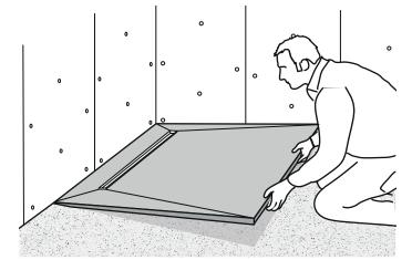
7) Position the shower base over the drain to make sure they are correctly aligned. (But don't remove the protective cover and force the nozzle in to the drain). Ensure any connections created are waterproof at this stage because it will not be possible to return to them once the unit is tiled. (You can do this by pouring water down the drain to check the seals).
