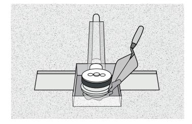
6) Lay the connected drain body and waste pipe into the channel and place a dab of mortar or cement based tile adhesive beneath the drain body to bring it level with the surrounding floor. Then infill around the connecting pipe to also bring this area level with the floor.
