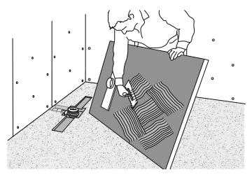
8) Comb out a continuous layer of cement-based single part flexible tile adhesive (such as **TileBacker Rapid Flex Adhesive**) to the underside of the shower base using a 10mm notched spreader. Keep the adhesive clear of the drain nozzle area.
