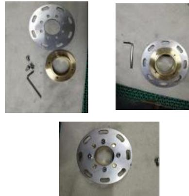
11. Fit the cover plate with copper ring over the stand pipe
