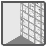
Timber grounds should be applied over poor surfaces, set approximately at 60cm vertically and 80cm horizontally as appropriate.
