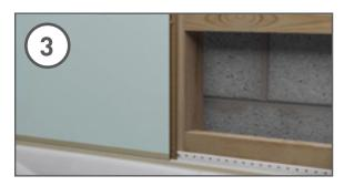
Fix through the back flange of the grooved edge with countersunk screws - the screw head should fit into the recess on the back of the tongue. Ensure that screws are turned until they are just under the flush to prevent any obstruction to the tongue of the next panel to be fitted.
