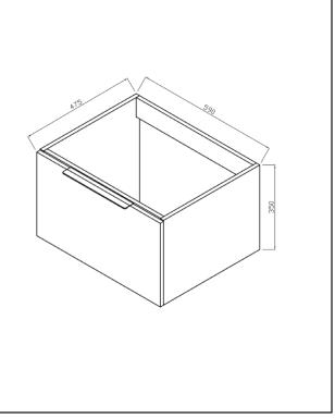
Dimensions (measurements in mm)
