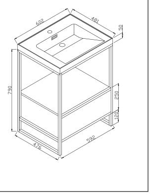
Dimensions (measurements in mm)
