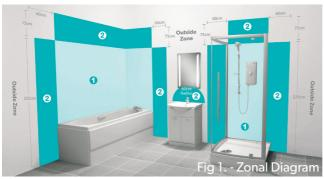
All installations must comply with quidelines which are based on a zonal concept and must be followed to ensure the safe installation of electrical appliances in the bathroom.
