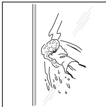
Step J Applying Silicone Sealant And Cleaning Seal from the top of the wall channel to the bottom on the INSIDE and Outside between the wall channel and the wall, and between the bottom profile and shower tray as shown. Wash down with clean warm water and a soft clean cloth or sponge. Please do not use bleach, alkaline or acid-based, aggressive or abrasive cleaning products.
