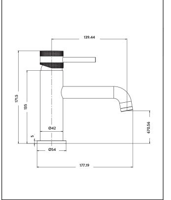
Dimensions (measurements in mm)
